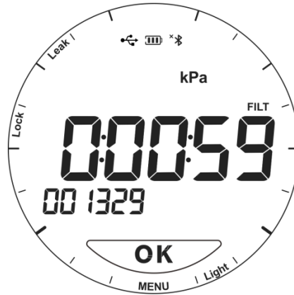
Figure 6 Pressure leak test setting interface
