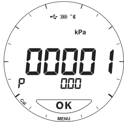
Figure23 Pressure calibration interface
